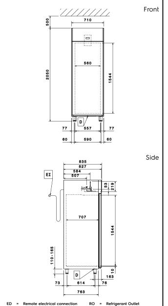
Remote electrical connection Electrical inlet (power) RO = Refrigerant Outlet EI
